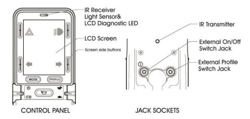
The actual design of this control system may vary depending on the specification and type of wheelchair you are working with. Refer to the wheelchair's documentation for exact details of the system you are working with.
